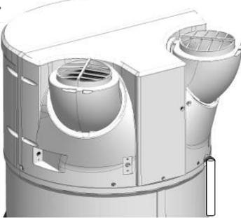
Depending on the humidity of the air, **up to 0.5l/h of condensates** may form. These condensates must not flow directly to the sewer, as the ammonia vapours discharged from the sewer could damage the fins of the heat exchanger and the components of the heat pump.
