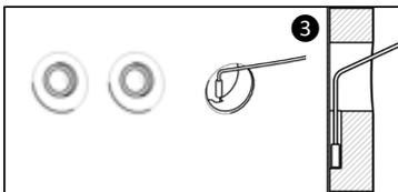
Insert the sensor into the chute ensuring that it is well positioned at the bottom of the housing.
