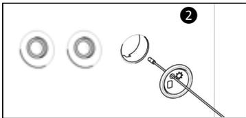
Push the temperature sensor through the plug (the plug has been drilled for this purpose).
