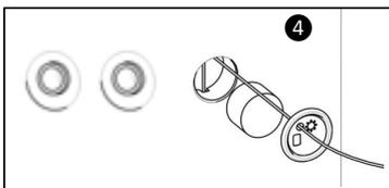
Put the foam back and insert the plug back into the product
