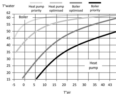
In addition, the Smart Energy function can be set with 4 different priority levels:
