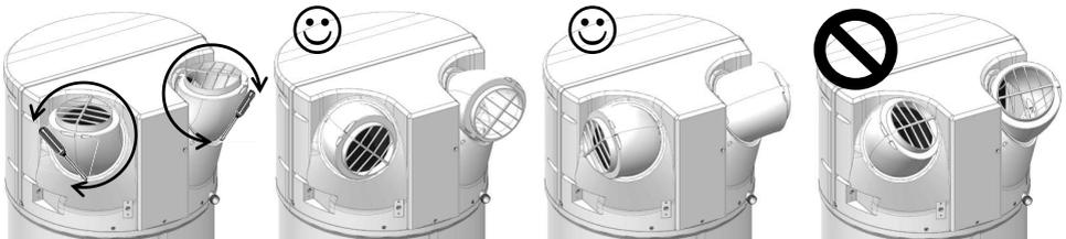
❶ Unscrew the vents' locking screws and rotate them to select the required direction
