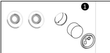
Remove the plug and foam from the housing next to the connections of the internal heat exchanger.
